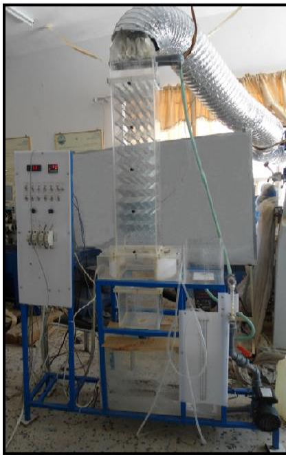
Figure (2) Experimental rig of forced draft counter flow water cooling tower.
